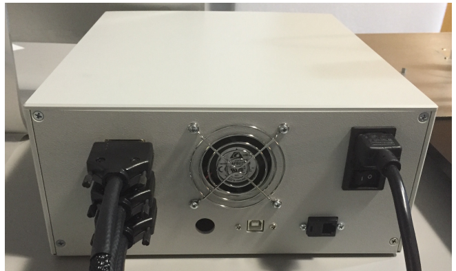
Positioning stage X, Y, and axis cables. These are interchangeable, and can be attached in any order.
