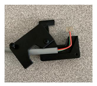
You can now remove the old micropipette by removing the RJ 11 wire assembly and dipping the piezo/micropipette end of the RJ 11 wire in acetone until the glue holding the micropipette is dissolved. Be careful to only dip the piezo and not the grey insulation on the RJ 11.
